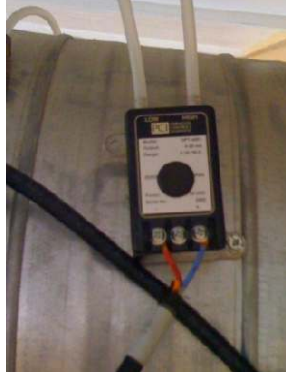
Figure 3.16 Differential Pressure Transducer for Air Flowrate
