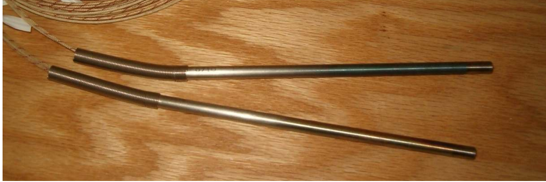
Figure 3.12 Exhaust RTD Sensors
